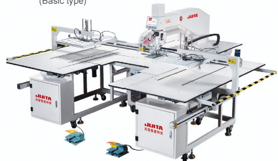
K10-90AWWJ 伸臂架机头360° 左右双送料带激光 Outstretched arm machine head rotate 360° seam Left and right double feeding with laser function
