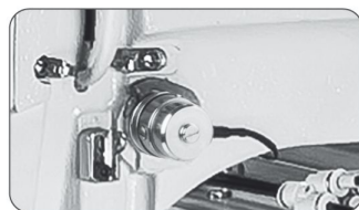
O—电子夹线器/电子压线松紧调节器 O—Electronic gripper Electronic crimping tension regulator
