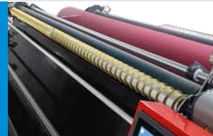
3*7MM METAL SPRING TYPE FABRIC FLATTENING BAR
