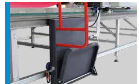
FOLDABLE OPERATOR PLATFORM WITH SAFETY BARRIER
