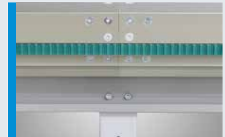
BOLT/PIM ARE USED AT RAIL JOINT / ENCODER BELT
