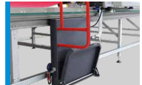
FOLDABLE OPERATOR PLATFORM WITH SAFETY BARRIER
