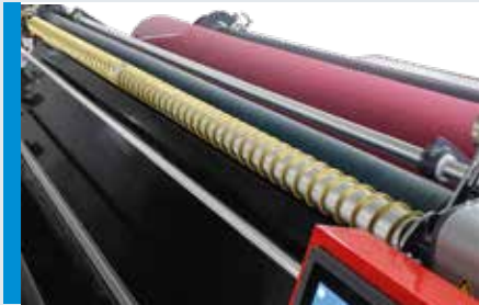
3*7MM METAL SPRING TYPE FABRIC FLATTENING BAR
