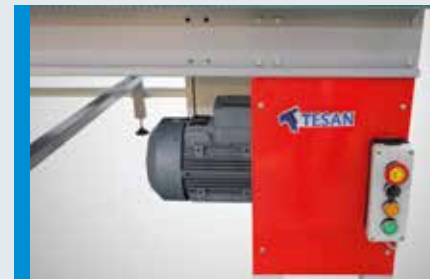
CONVEYOR MOTOR AND CONTROL BUTTON
