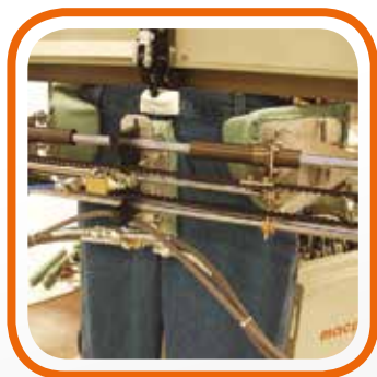
Stiro a vapore contemporaneo delle tasche e patella Contemporary pressing of flap and pockets
